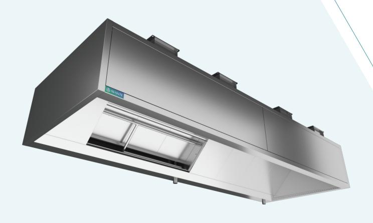
Avante-EF-WW is an extract-only canopy with Water Wash, equipped with front and side induction nozzles to contain and extract fumes and heat within the hood area, thereby improving the extract efficiency and working conditions. The front section is equipped with a fan that uses the ambient air from the surrounding area to supply air through the induction nozzles.
