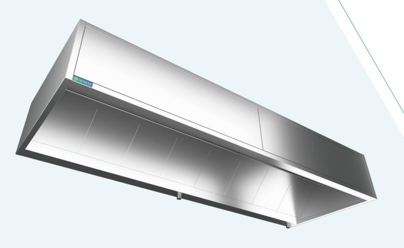
Avante-EF-WM is an extract-only canopy with Water Mist, equipped with front and side induction nozzles to contain and extract fumes and heat within the hood area, thereby improving the extract efficiency and working conditions. The front section is equipped with a fan that uses the ambient air from the surrounding area to supply air through the induction nozzles.
